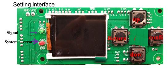
There are four first level menus: system setting, operation mode, display setting and factory setting, which are simple to operate and fast to respond.
