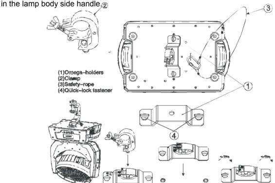
Warning: Do not use the hand of the LED moving head to up and down or fix.
