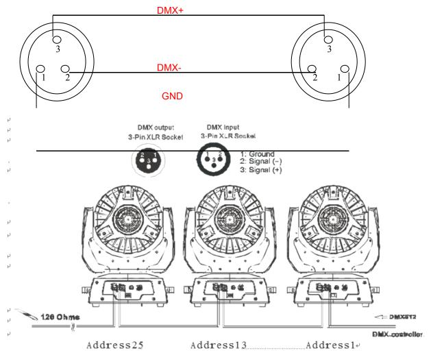
Connecting DMX512 digital signal, Please using high quality screen line to connect it, for fear interfering.
