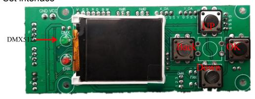
There are system settings, running mode, display settings, factory set up four first-level menu, simple operation, fast response..
